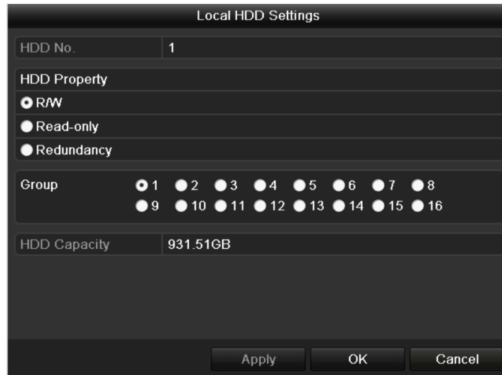
Figure 10. 15 Local HDD Settings Interface
